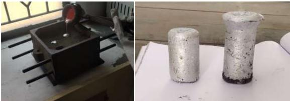
Figure 4: MOULD CAVITY FILLED WITH MOLTEN METAL Figure 5: FINAL PRODUCT
